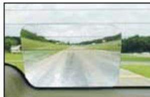
**THE TYPES OF BACKUP AIDS** With camera systems, left, a monitor shows obstacles in the driver's blind spot; this one mounts under the rear-view mirror. A plastic fish-eye lens, right, also reduces the rear blind spot. A sensor unit, center, sits on the dashboard. It beeps and lights up to help the driver park.
